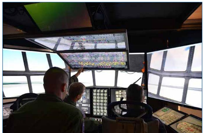
working to complete the C-130H3 variant in late summer 2017. The device is totally reconfigurable with the press of a button, allowing a single MMCT to be capable of training H2, H3 and LC130 at all sites.
